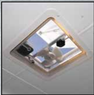
Roof Vent with Exhaust Fan
